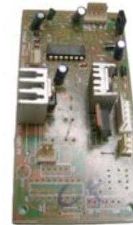
*Hybrid solar lantern circuit board using surface mount technology - India (circa 2012)*
