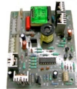
*Solar lantern circuit board based on 'through-hole technology' - India (circa 1998)*
